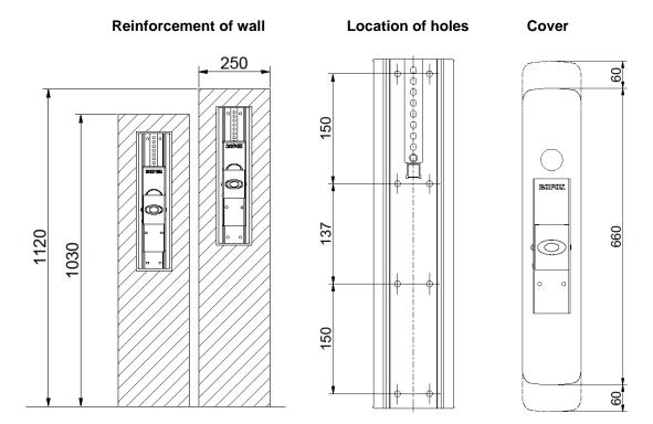
The hatched area is the minimum area for reinforcement of the wall. Reinforcement from floor to ceiling is advisable. The holes are measured on the basis of the upper holes of the wall bracket and the location depends of the type of toilet support arm to be used. It must be ensured that the cover can move 60mm upward and downward.
